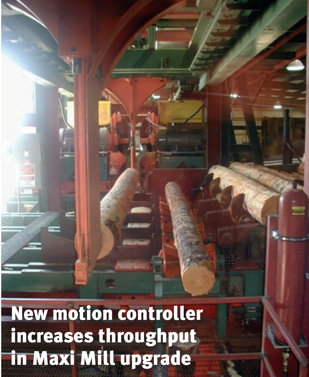
Maxi Mill end doggers (left) and chargers (center right) move the logs
